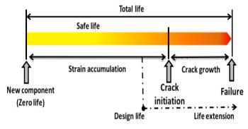
Fig. 3 Creep life span of hot section components due to deformation
